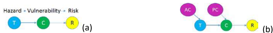
Figure 1. Elemental Bayesian Network representations of Risk Assessment (a) and or Risk Assessment and Management (b).
